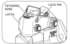
• Open the latch by rotating the latch assembly up toward the vehicle until the latch is in its most upright position, then release the lock handle. (Figure 17 and 18).
