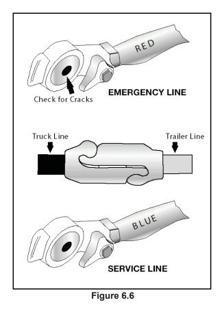
If you do cross the air-lines, supply air will be sent to the service line instead of going to charge the trailer air tanks. Air will not be available to release the trailer spring brakes (parking brakes). If the spring brakes don't release when you push the trailer air supply control, check the air-line connections.
