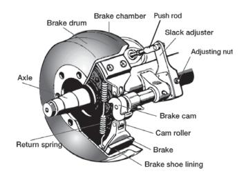
Brake drums are located on each end of the vehicle's axles. The wheels are bolted to the drums. The braking mechanism is inside the drum. To stop, the brake shoes and linings are pushed against the inside of the drum. This causes friction which slows the vehicle and creates heat. The amount of heat that a drum can take without damage depends on how hard and how long the brakes are used. Too much heat can make the brakes stop working.
